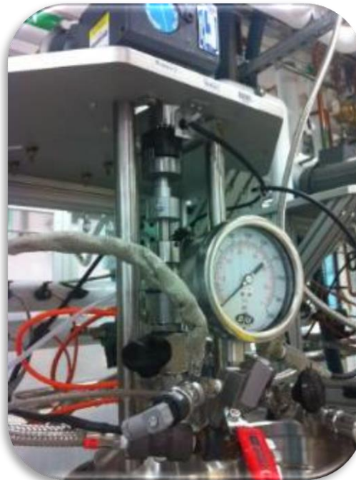
Self-sealing packed gland drive
