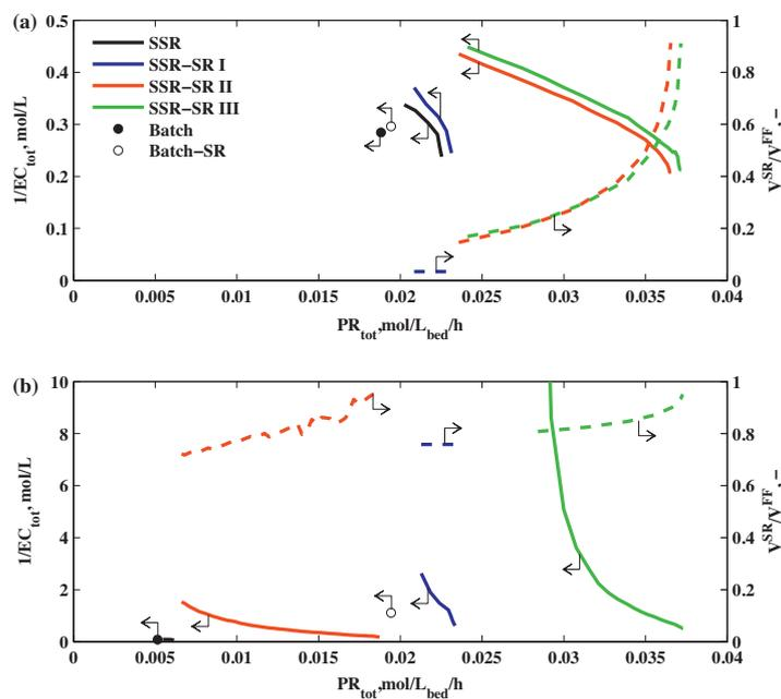
**Fig. 6.** Pareto frontiers (solid lines) and the relative amount of solvent removed (dashed lines) for different process modes and configurations. Solvent removal unit is the limiting step (concentration limits B). (a)  $c^{FF} = 1.35$  mol/L; (b)  $c^{FF} = 0.34$  mol/L.
