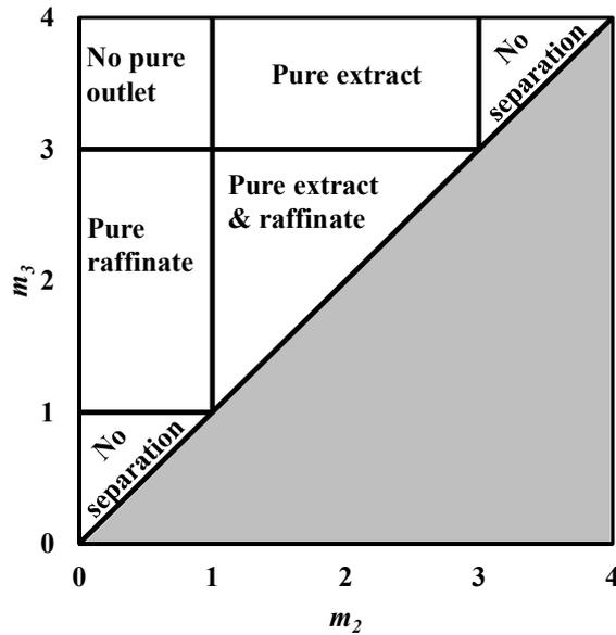
Figure 6 The purities of product streams at different operation region on the  $(m_2, m_3)$  plane for a system with linear isotherms with  $H_A = 3$  and  $H_B = 1$  (adapted from [52]).
