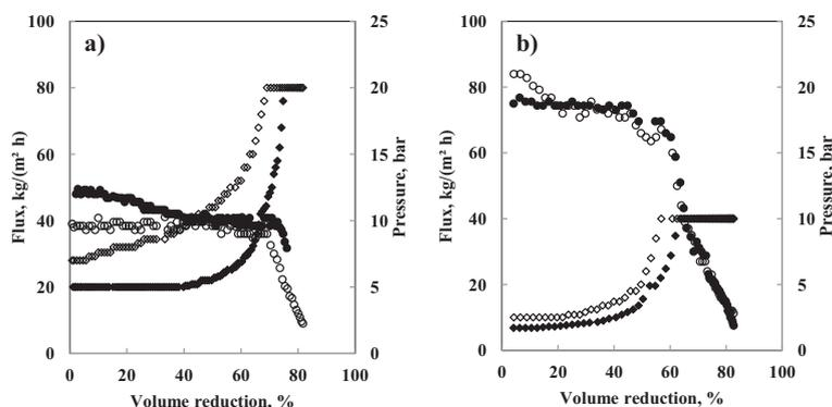
**Fig. 2 – Pressure (diamonds) and flux (circles) in the ultrafiltration of HW soda black liquor (open symbols) and SW soda black liquor (filled symbols) using (a) the NP010 (1 kDa) and (b) the UP010 (10 kDa) membranes. Temperature was 60 °C and cross flow velocity about 2.3 m/s.**
