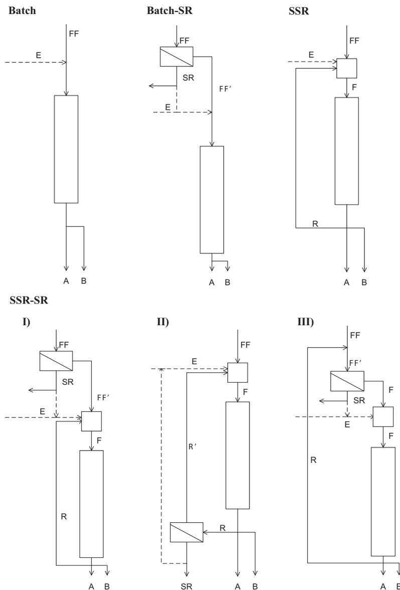
**Fig. 1.** Chromatographic process configurations investigated. Principles of SSR–SR schemes: (I) Solvent removal from the fresh feed; (II) solvent removal from the recycle stream; (III) solvent removal from the column feed. FF=fresh feed, F=feed to the column, R=recycle fraction, SR=removed solvent, E=eluent. A and B are the product fractions.
