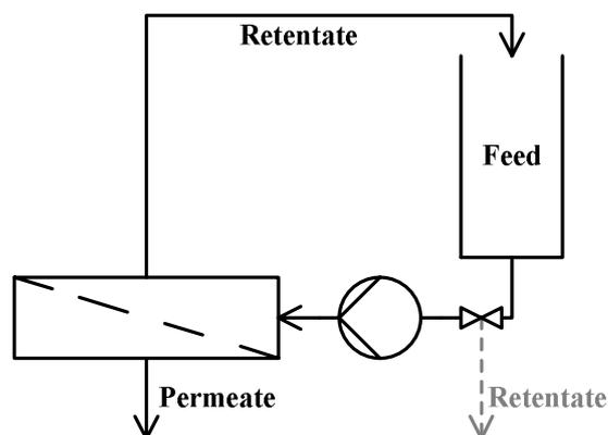
Figure 12 Simplified scheme of the membrane filtration equipment applied.
