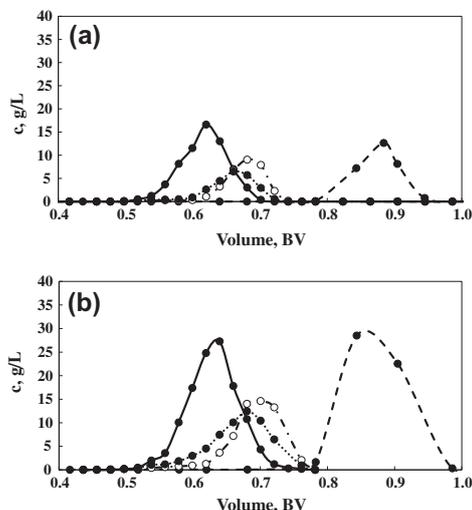
**Fig. 2.** Outlet profiles in SW soda black liquor fractionation using Sephadex G-10: isosaccharinic acids (solid line); volatile acids (dash-dot line); other acids (dotted line); NaOH (dashed line). (a) Feed concentration 10 wt% d.s. (b) Feed concentration 25 wt% d.s.  $H_{\text{bed}} = 20$  cm,  $D_{\text{bed}} = 2.5$  cm,  $V_{\text{inj}} = 0.08$  BV,  $\dot{V} = 0.61$  BV/h,  $T = 50$  °C. Acid concentrations are determined using CE and NaOH concentrations are estimated based on pH.
