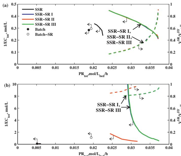
Fig. 7. Pareto frontiers (solid lines) and the relative amount of solvent removed (dashed lines) for different process modes and configurations. Column feed is the limiting step (concentration limits D). (a)  $c^{FF} = 1.35$  mol/L; (b)  $c^{FF} = 0.34$  mol/L.
