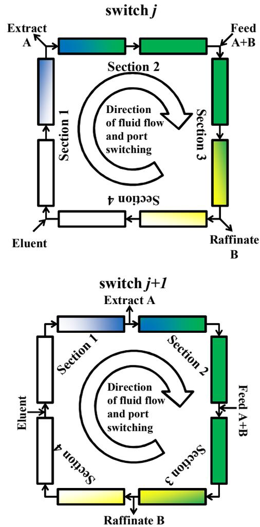
Figure 5 A simplified scheme of a four-zone SMB (adapted from [51]).
