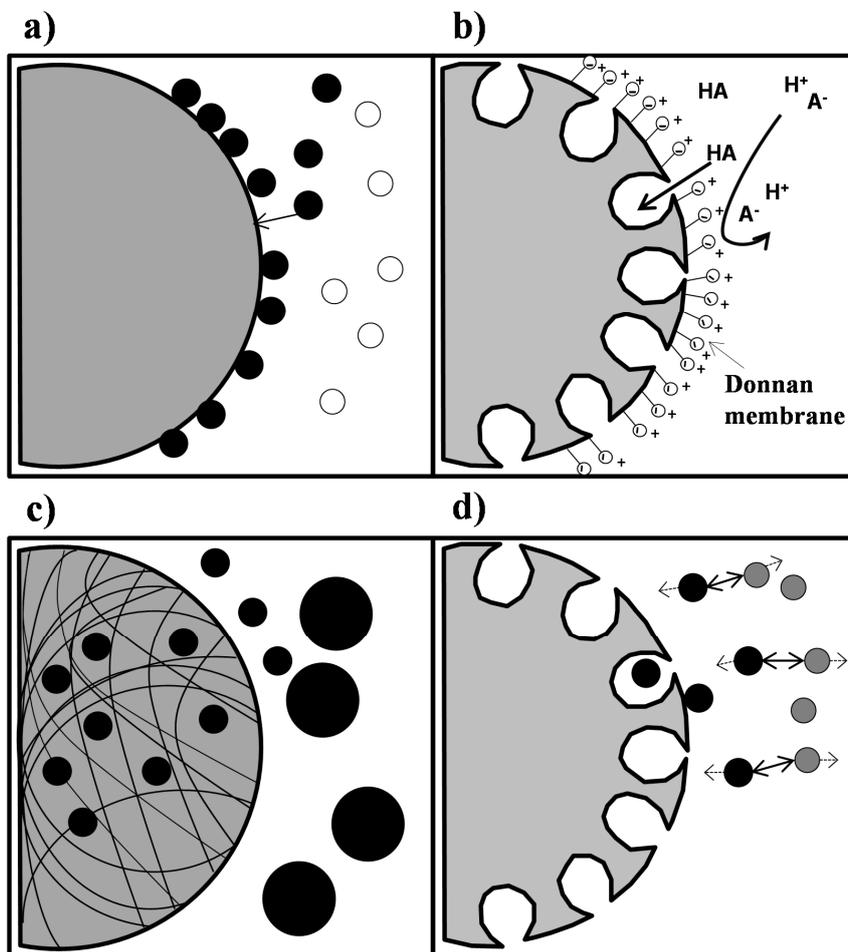
Figure 2 Examples of separation mechanisms in chromatography: a) adsorption, b) ion-exclusion, c) size-exclusion, d) salting out.
