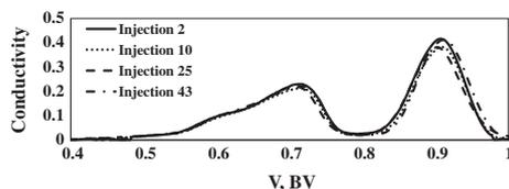
Fig. 6. Conductivity profiles of 4 randomly chosen injections recorded during 44 consecutive pulse injections ( $V_{inj}$  8% of BV) of HW soda black liquor.  $H_{bed} = 11.5$  cm,  $D_{bed} = 1.5$  cm,  $V = 1$  BV/h,  $T = 50$  °C.
