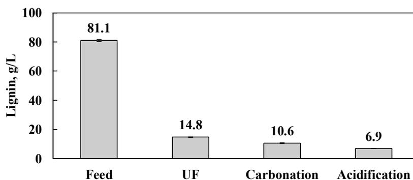
Figure 14 Concentration of lignin in SW soda black liquor after different process steps: UF using the NP010 membrane, carbonation (final pH 9), and sulphuric acid precipitation (final pH 2.5). The error bars show the deviation in the results of parallel samples.
