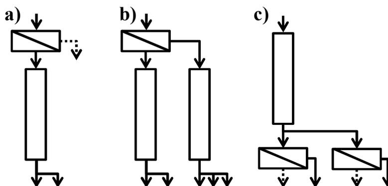
Figure 9 Different ways of combining of chromatographic and membrane separations in a tandem process: a) Pre-treatment using membrane filtration, b) Fractionation of a multicomponent mixture, c) RO for concentration of the products from chromatographic separation.
