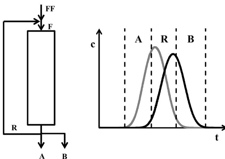
Figure 4 The principle of SSR chromatography. FF = Fresh feed, F = feed to column, A = first product fraction, B = second product fraction, R = recycle fraction.
