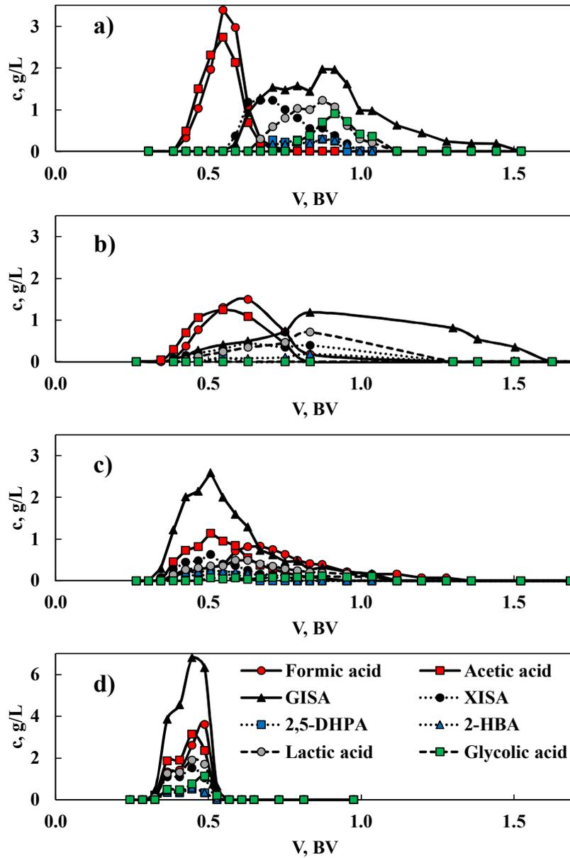
Figure 18 Fractionation of SW soda black liquor (pre-treated by UF, 10% TDS) using a) SAC resin (Finex CS16GC) in  $\text{Ca}^{2+}$  form, b) SAC resin (Finex CS16GC) in  $\text{Ba}^{2+}$  form, c) WAC resin (Finex CA16GC) in  $\text{Ca}^{2+}$  form, d) WAC resin (Finex CA16GC) in  $\text{Na}^{+}$  form.  $V_{inj} = 0.08$  BV, eluent flow rate 0.6 BV/h. The acids are in their Na salt form.
