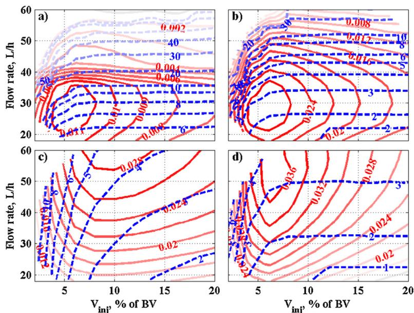
**Fig. 5.** Process performance of SSR (a), SSR–SR I (b), SSR–SR II (c), and SSR–SR III (d) when concentration limits  $C$  (see Table 1) are applied and  $c^{FF} = 0.68$  mol/L. Red solid lines: productivity (mol/L<sub>bed</sub>/h); blue dashed lines: eluent consumption (L/mol). Removed solvent is re-used as eluent. (For interpretation of the references to colour in this figure legend, the reader is referred to the web version of the article.)
