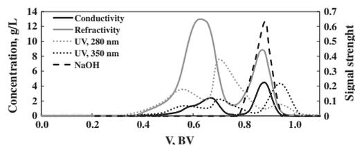
Fig. 1. Chromatograms obtained using the online detectors during fractionation of SW soda black liquor (d.s. 10%) using Sephadex G-10. Concentration of NaOH is estimated base on pH measured off-line.  $H_{\text{bed}} = 20 \text{ cm}$ ,  $D_{\text{bed}} = 2.5 \text{ cm}$ ,  $V_{\text{inj}} = 0.08 \text{ BV}$ ,  $V = 0.61 \text{ BV/h}$ .
