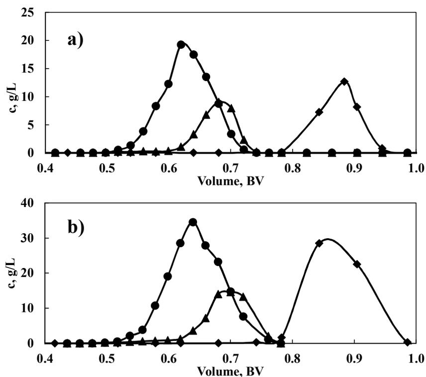
Figure 15 Fractionation of SW soda black liquor using Sephadex G-10 SEC gel. Outlet concentration of hydroxy acids (circles), volatile acids (triangles), and NaOH (diamonds). Feed concentration: a) 10% TDS; b) 25% TDS.  $V_{inj} = 0.08$  BV, eluent flow rate 0.6 BV/h. Lines are to guide the eye.
