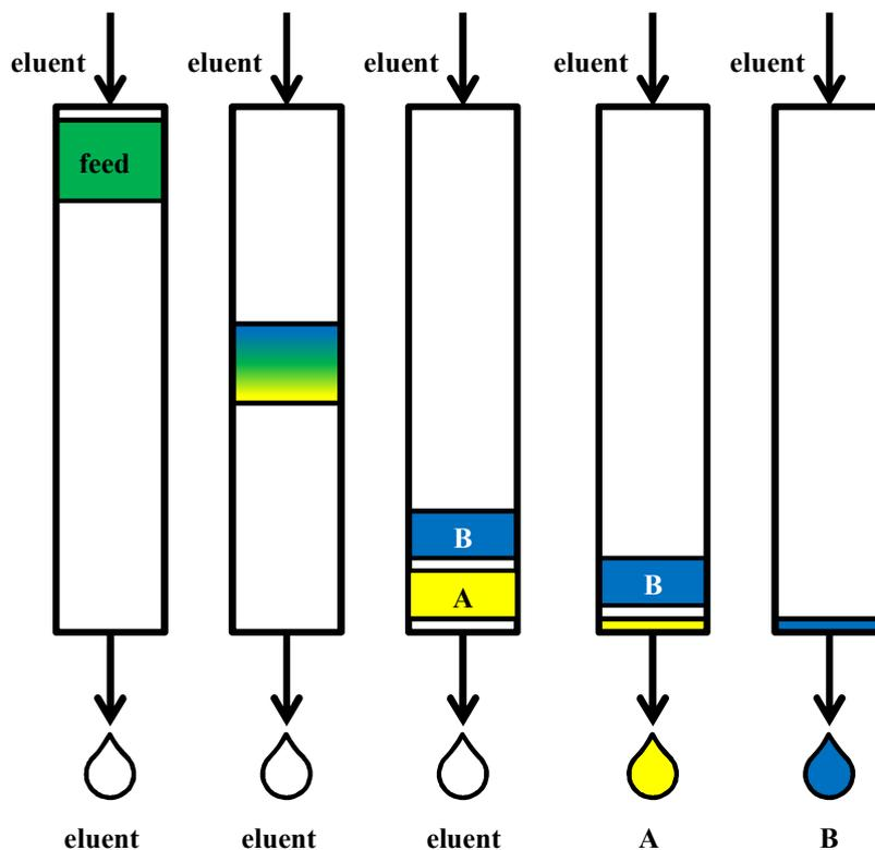
Figure 3 Chromatographic separation of a binary mixture of compounds A and B in batch mode. Separation occurs at ideal conditions and both components possess linear isotherms.
