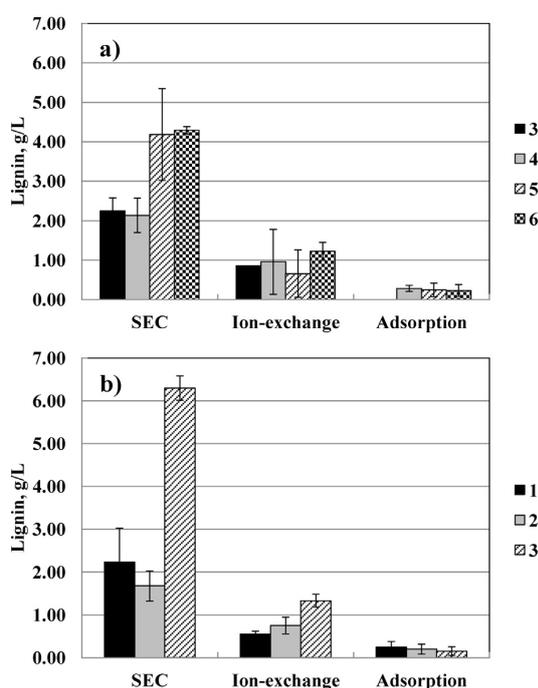
**Fig. 4 – Concentration of lignin in the fractions after the different process steps: (a) HW soda black liquor and (b) SW soda black liquor. The NP010 membrane was applied for pre-treatment.**
