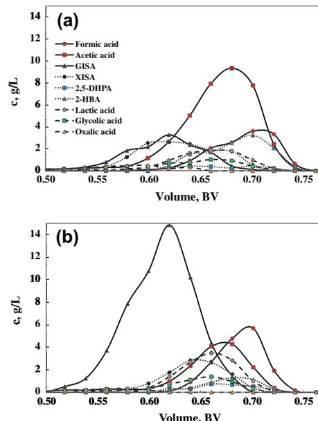
**Fig. 4.** Concentrations of individual acids in the chromatograms displayed in Figs. 2a and 3a. (a) SW soda black liquor and (b) HW soda black liquor. NaOH is not shown but elutes after the acids (see Figs. 2 and 3). Sephadex G-10 column, feed concentration 10 wt% d.s.,  $H_{\text{bed}} = 20$  cm,  $D_{\text{bed}} = 2.5$  cm,  $V_{\text{inj}} = 0.08$  BV,  $\dot{V} = 0.61$  BV/h,  $T = 50$  °C.
