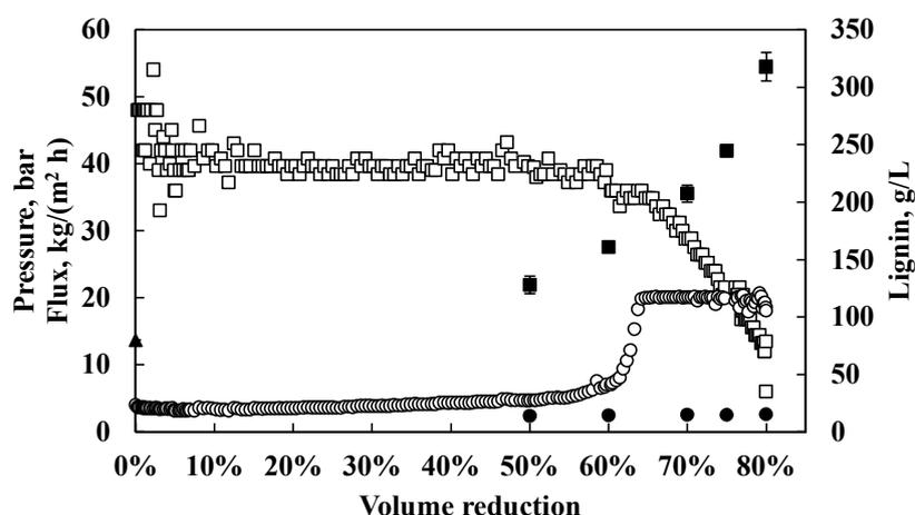
Figure 13 UF of SW soda black liquor using the NP010 membrane. Pressure (○), Flux (□), the concentration of lignin in the feed (▲), permeate (●) and retentate (■).  $T = 60\text{ }^{\circ}\text{C}$ , cross-flow velocity 2.3 m/s.
