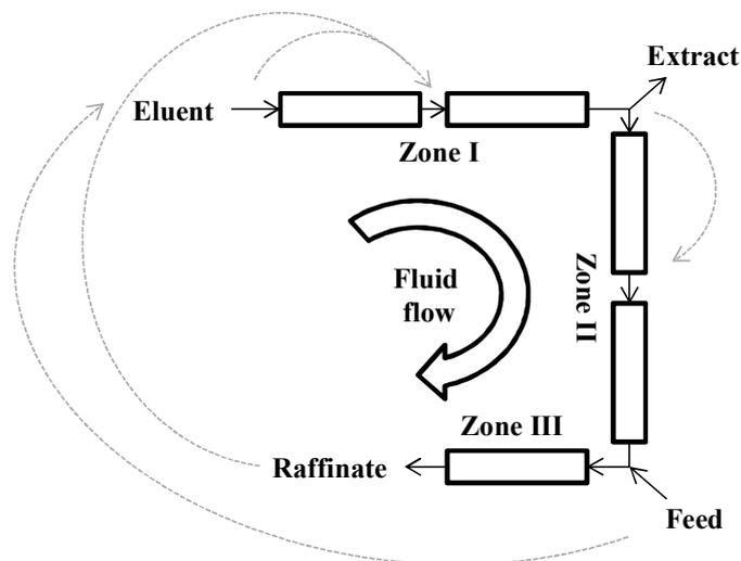
Figure 11 SMB configuration used in the separation of NaOH and hydroxy acids.
