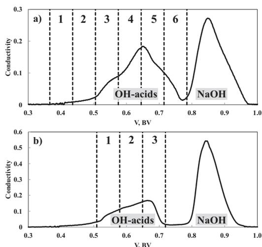
**Fig. 3 – Fractionation of hydroxy acids of (a) HW soda black liquor and (b) SW soda black liquor using Sephadex G-10.  $H_{bed} = 40.7$  cm,  $D_{bed} = 5$  cm,  $V_{inj} = 0.1$  BV; eluent flow rate  $0.6$  BV/h.**
