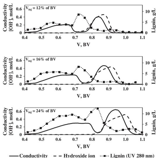
Fig. 5. Chromatograms obtained using different injection volumes of HW soda black liquor (10% d.s.).  $H_{\text{bed}} = 20$  cm,  $D_{\text{bed}} = 2.5$  cm,  $V = 0.61$  BV/h,  $T = 50$  °C.
