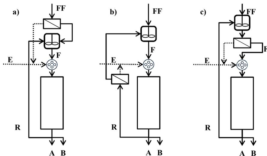
Figure 10 Different positions of the solvent removal unit in an SSR-SR process: a) concentration of fresh feed, b) concentration of recycle fraction, c) concentration of the mixed feed. (Adapted from [24].)
