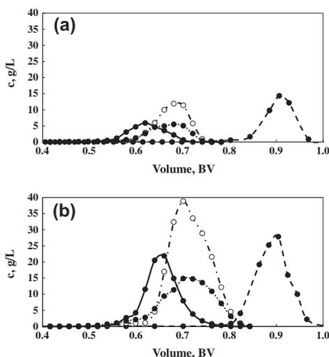
**Fig. 3.** Outlet profiles in HW soda black liquor fractionation using Sephadex G-10: isosaccharinic acids (solid line); volatile acids (dash-dot line); other acids (dotted line); NaOH (dashed line). (a) Feed concentration 10 wt% d.s. (b) Feed concentration 25 wt% d.s.  $H_{\text{bed}} = 20$  cm,  $D_{\text{bed}} = 2.5$  cm,  $V_{\text{inj}} = 0.08$  BV,  $\dot{V} = 0.61$  BV/h,  $T = 50$  °C. Acid concentrations are determined using CE and NaOH concentrations are estimated based on pH.
