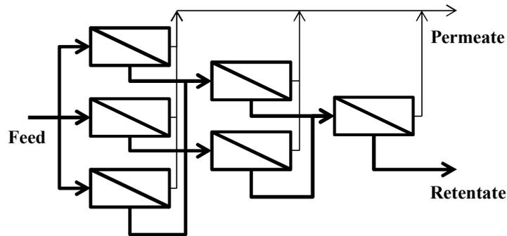
Figure 8 A single-pass membrane cascade with a “Christmas tree” design.
