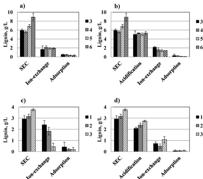
Fig. 5 – Lignin concentration in the fractions after the different process steps: (a) HW soda black liquor without acidification; (b) HW soda black liquor with acidification; (c) SW soda black liquor without acidification; and (d) SW soda black liquor with acidification. The UP010 membrane was applied for pre-treatment.
