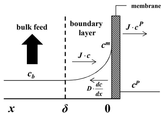
Figure 7 Concentration polarisation in membrane filtration (adapted from [84]).
