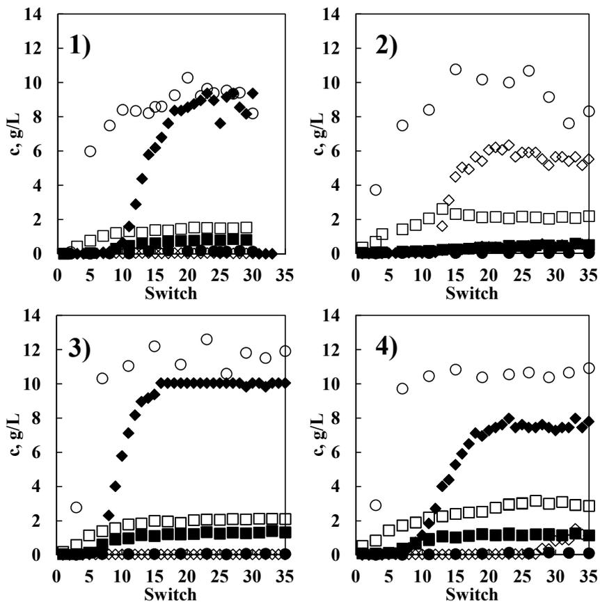
Figure 17 Concentration of NaOH (diamonds), acids (circles), and lignin (squares) in the extract (closed symbols) and raffinate (open symbols). The parameters for each run are presented in Table 3 and Fig. 16.
