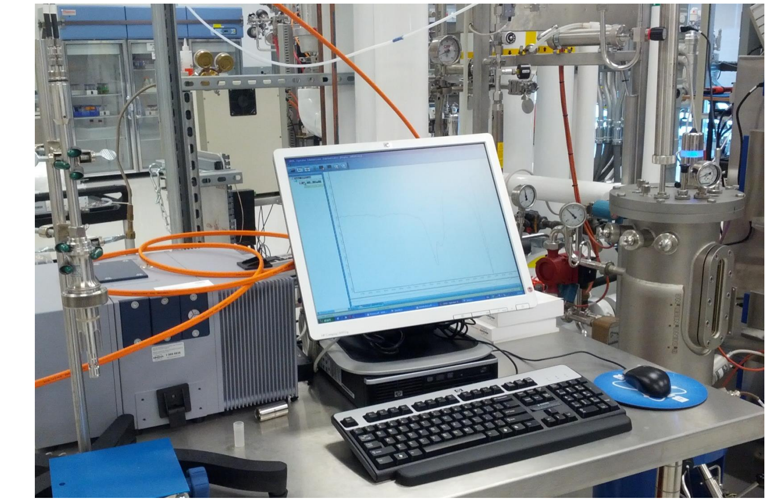
Figure 3: Bruker Optics Matrix-F FT-NIR with Flex Transflexion probe Linear and Exponential Fed-Batch Fermentation
