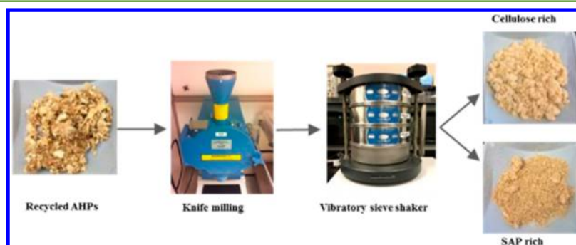
Figure 2. Mechanical removal of SAP from AHPs.
